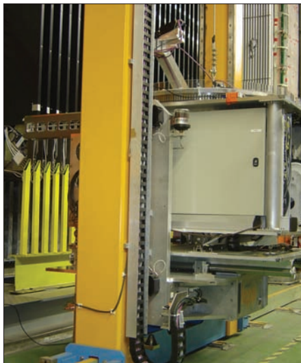
Fig. 3. The brick manipulator system approaching a wall for brick loading.
